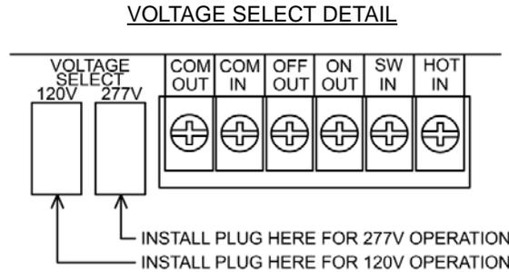
**CAUTION:** Failure to install the Voltage Selector Plug will prevent system operation. Installing the Voltage Selector Plug in the position that does not match the actual AC input line voltage will damage the unit, void the warranty and may cause a dangerous or unsafe condition.
